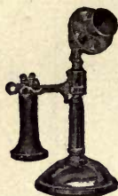
FIGURE 225.—A PORTABLE TELEPHONE RECEIVER AND TRANSMITTER.
